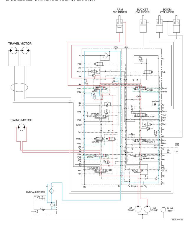
When the swing and arm functions are operated simultaneously, the swing spool and arm spools in the main control valve are moved to the functional position by the pilot oil pressure from the remote control valve.
