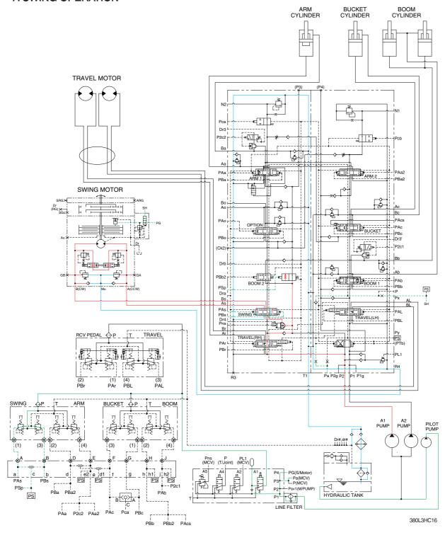
When the LH control lever is pushed left or right, the swing spool in the main control valve is moved to the left or right swing position by the pilot oil pressure from the remote control valve.
